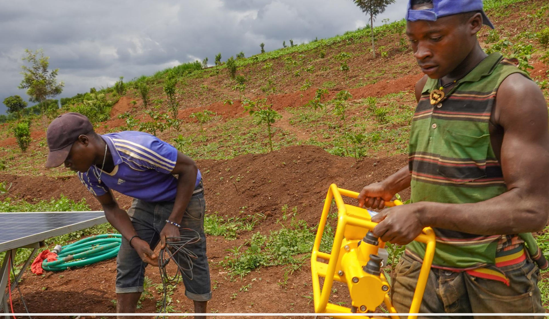
0.5 HP sunlight pump : Lightweight (14 kg) for transport where needed
